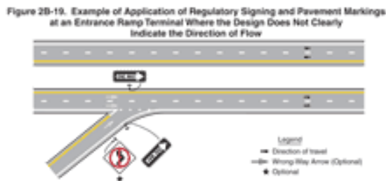
Figure 2B-19 Example of Application of Regulatory Signing and Pavement Markings at an Entrance Ramp Terminal Where the Design Does Not Clearly Indicate the Direction of Flow
