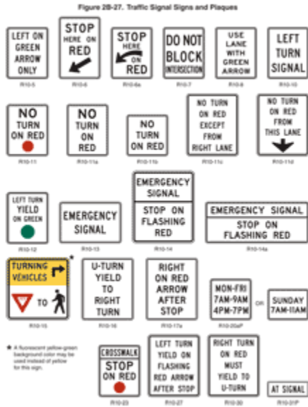
Figure 2B-27 Traffic Signal Signs and Plaques
