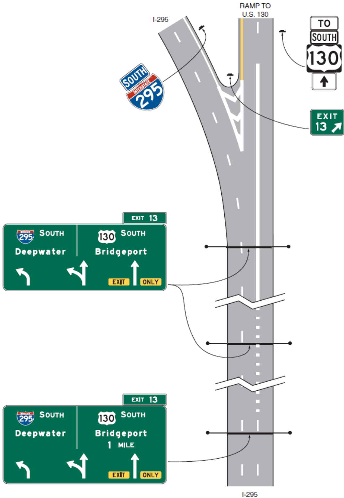
Figure 2E-5. Overhead Arrow-per-Lane Guide Signs for a Two-Lane Exit to the Right with an Option Lane (Through Lanes Curve to the Left)
