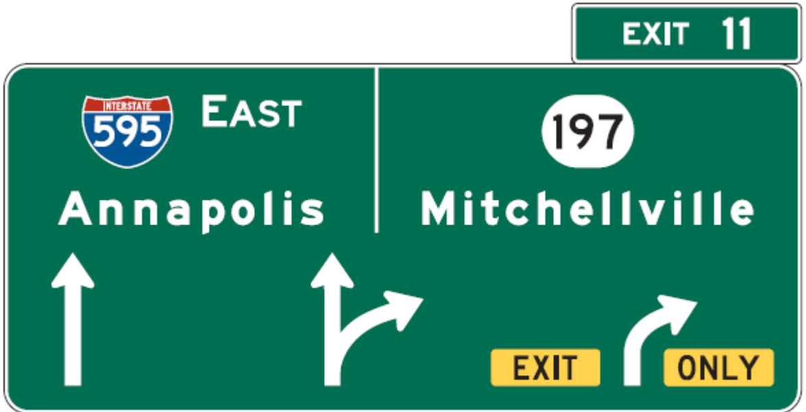
199 Figure 2E-3. Overhead Arrow-per-Lane Guide Sign for a Multi-Lane Exit with an Option Lane
