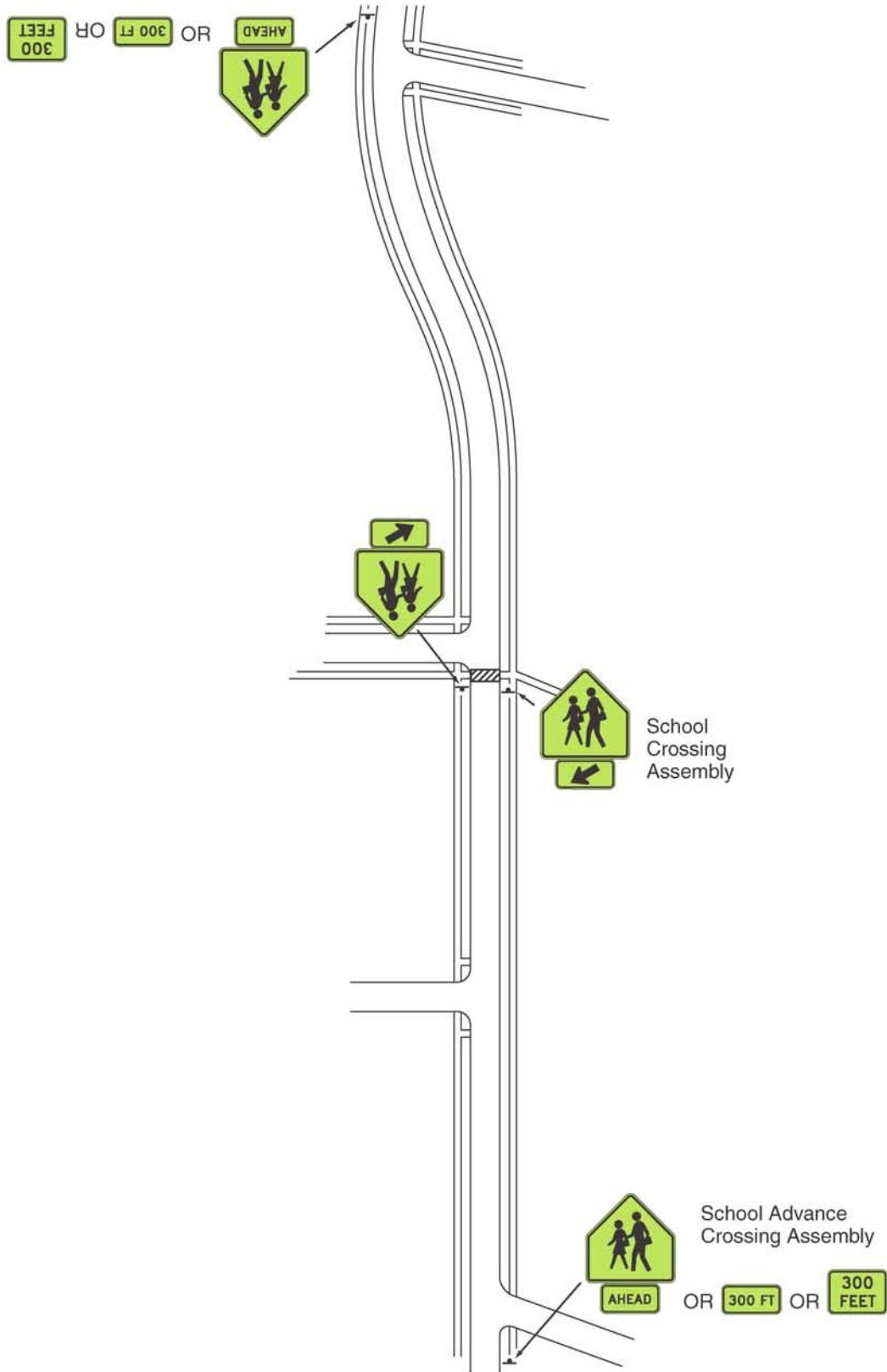
Figure 7B-3. Example of Signing for a School Crossing Outside a School Zone
