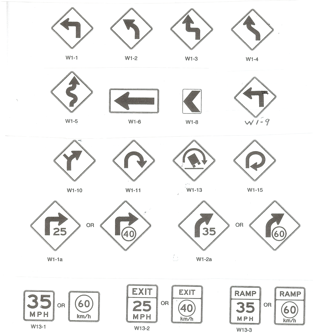
Revised Figure 2C-1. Horizontal Alignment Signs
