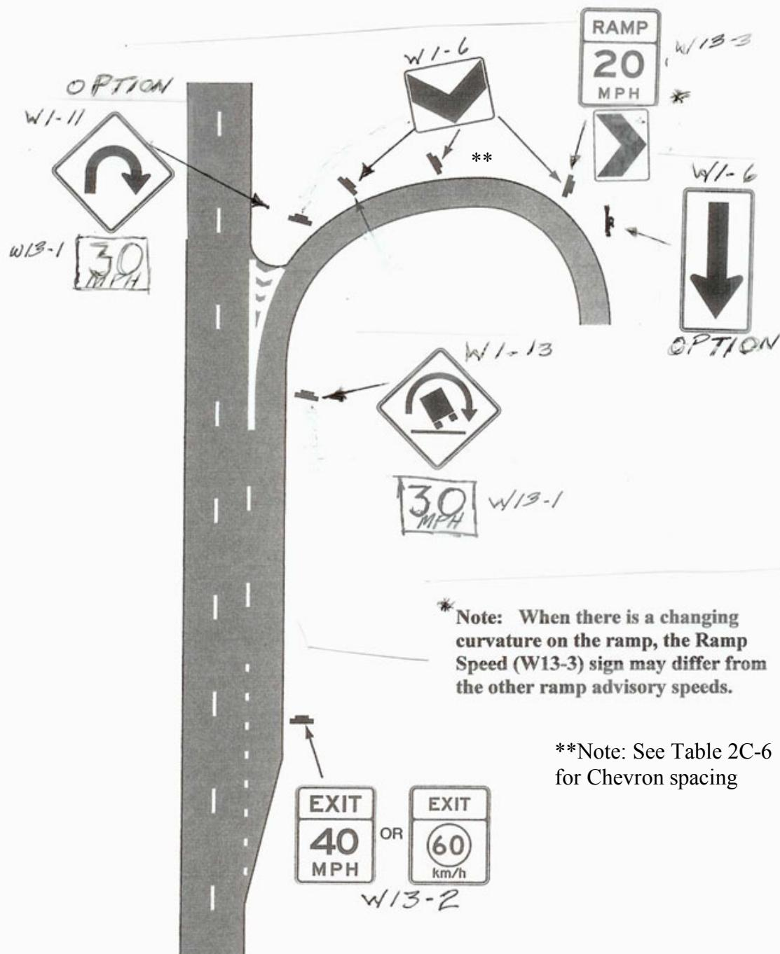
Add a new Figure 2C-X. Example of Signing for a Turn to illustrate the application of optional signing addressed in Sections 2C.07, 2C.09, 2C.10 and 2C.12.
