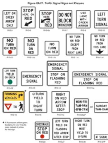
Figure 2B-27 Traffic Signal Signs and Plaques
