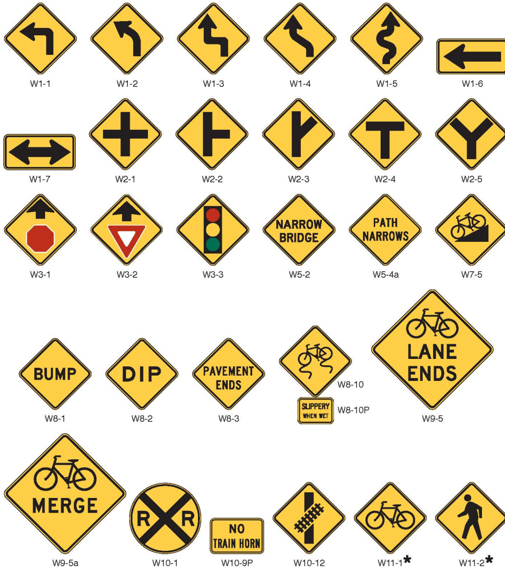
Figure 9C-1. Warning Signs and Plaques and Object Markers for Bicycle Facilities (Sheet 1 of 2)
