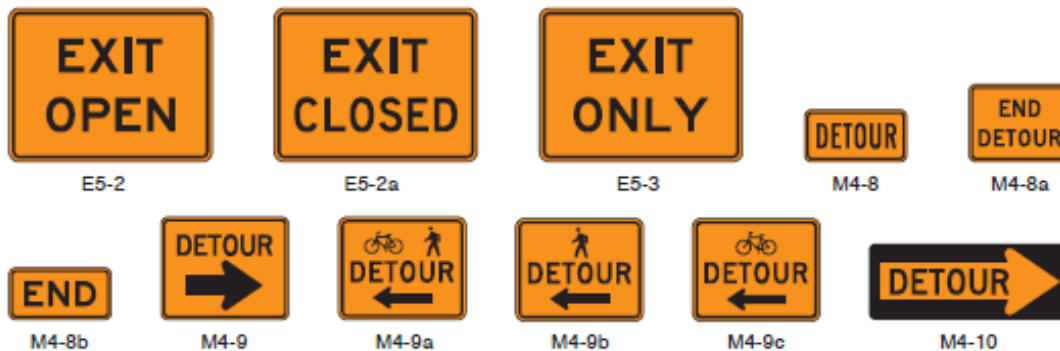
Figure 6I-1. Exit Open and Closed and Detour Signs
