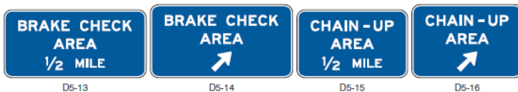
Figure 2I-6. Brake Check Area and Chain-Up Area Signs
