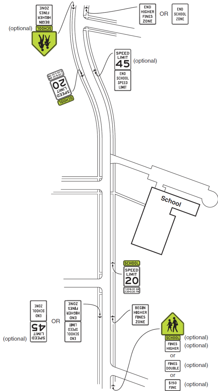
Figure 7B-3. Example of Signing for a Higher Fines School Zone with a School Speed Limit
