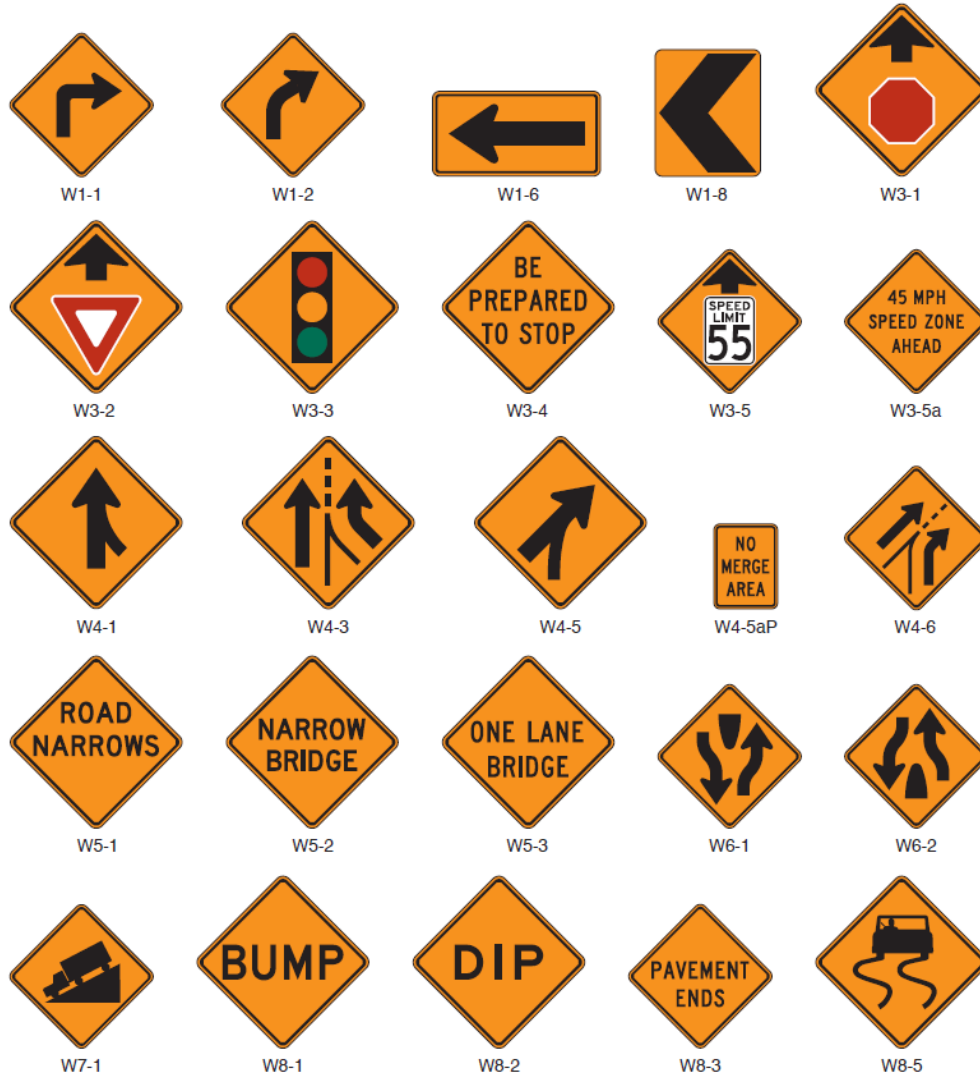
Figure 6H-1. Examples of Other Warning Signs Used in TTC Zones (Sheet 1 of 2)
