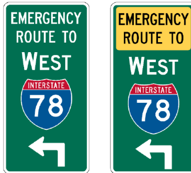
Examples of guide signs for rerouting
