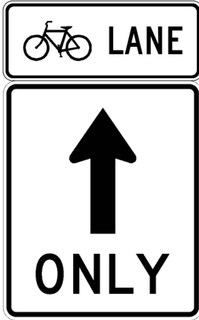
R3-5hP (30" x 12") mounted above R3-5a (bicyclists go straight in that lane)
