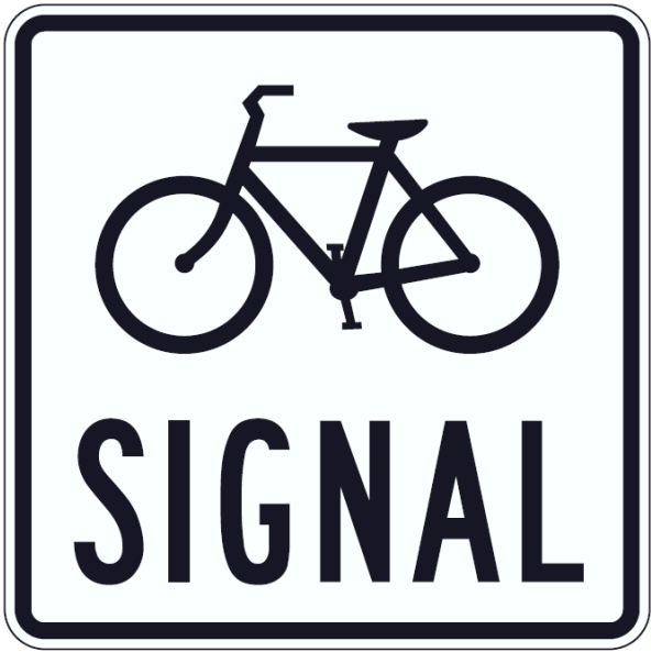
Bicycle Signal (R10-xx) sign - 24" x 24" 10" symbol, 6" B text (design could also be used for a 6" x 6" size under 4" near-side indications with a 2.5" symbol and 1.5" B text)
